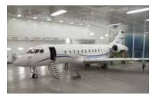
Air in a crossdraft booth flows from end to end, matching the natural flow of air across the aircraft. This provides excellent quality finishes.
