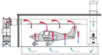
Downdraft aircraft booths can be designed for a specific plane to optimize the airflow design and overall efficiency of the system. This is especially true when using a booth for similar size and shaped aircraft. For the most economical design, a downdraft booth should be incorporated early into your facility's design process.
