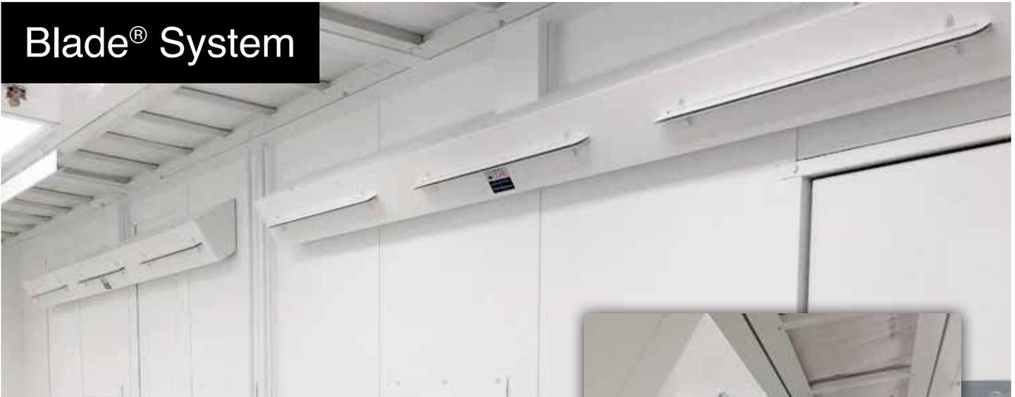
The Blade option for GFS' AdvanceCure System improves upon the class-leading performance of the standard nozzle system. Tested by paint companies, AdvanceCure Blade® provides premium performance and reduced maintenance, with no need to move or clean nozzles. The exclusive air-knife design enables the precise direction of air through small slits in the module. The Blade option can be added to most I-Series horizontal AdvanceCure models.
