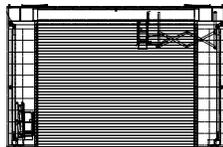
Roll-up doors are available in galvanized stainless steel and aluminum. Finishes range from 21 standard colors to 172 premium colors, or color-matched to customer specifications, as well as colored, anodized aluminum.
