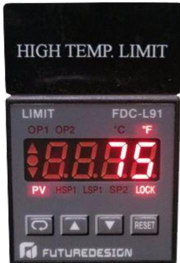
1. With the burner on, push and hold the **RESET** button on the high temperature limit until the **LOCK** light turns off.
