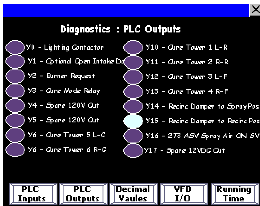
Figure 21. PLC Outputs screen
